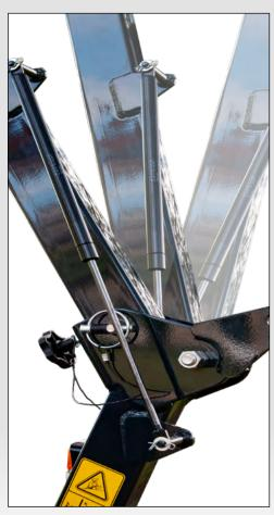
Assisted foldable ROPS which can drop down to allow for reduced space storage access.
